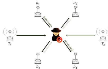
**Figure 1:** A bistatic radar network consisting of 2 radar transmitters  $T_1$ ,  $T_2$  and 4 radar receivers  $R_1$ ,  $R_2$ ,  $R_3$ ,  $R_4$ . Each transmitter-receiver pair operates as a bistatic radar.
