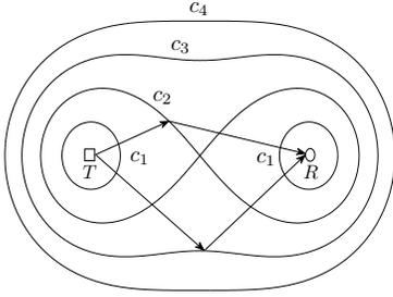
**Figure 2: Bistatic radar SNR contours as Cassini ovals with foci at BR transmitter  $T$  and receiver  $R$  for distance products:  $c_1 < c_2 < c_3 < c_4$ .**
