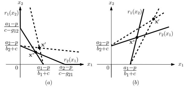
**Figure 5:** For Stage II for two users, the unique UDE  $\mathbf{x}^*$  is achieved at the intersection of the best response functions (bold lines): (a)  $\frac{g_{12}-c}{b_1+c} \in (-1, 0)$ ,  $\frac{g_{21}-c}{b_2+c} \in (-1, 0)$ ; (b)  $\frac{g_{12}-c}{b_1+c} \in (0, 1)$ ,  $\frac{g_{21}-c}{b_2+c} \in (0, 1)$ . When  $g_{12} = g_{21}$  increases, the UDE  $\mathbf{x}^*$  moves to  $\mathbf{x}'$ .
